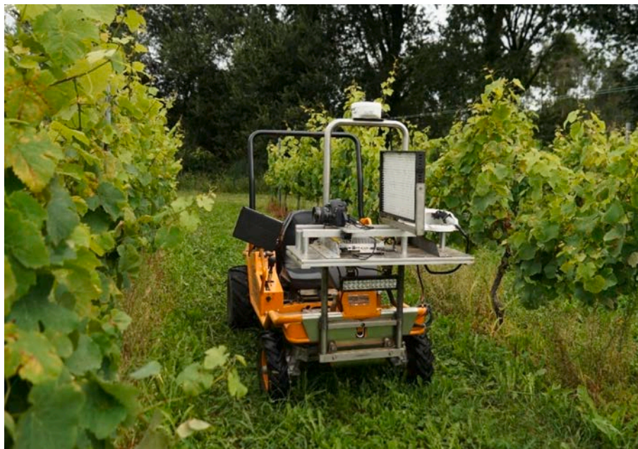
Fig. 2. Mobile platform used for taking the images on-the-go in the vineyard.
