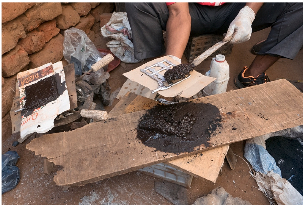
Fig. 3. Fabricated lead grids being coated in lead oxide paste and dried over a charcoal cooking stove during the informal lead-acid battery recycling process, described in detail in the supporting information.
