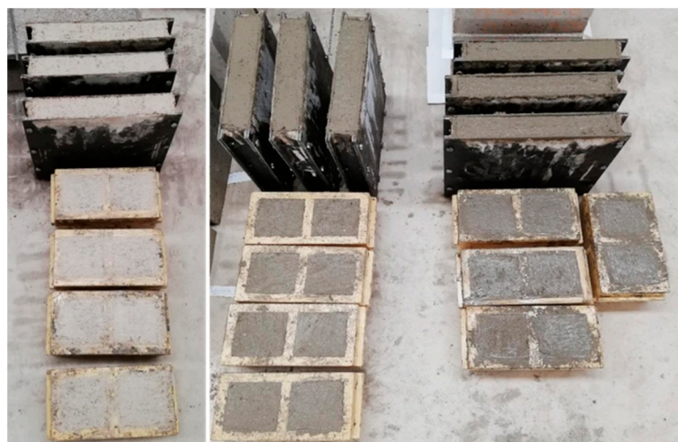
Figure 3. Curing of mortar samples (0.30 m × 0.30 m × 0.05 m).
