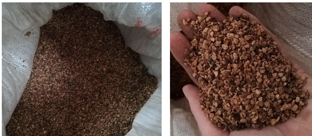
Figure 2. GOSs used into dope mortar.
