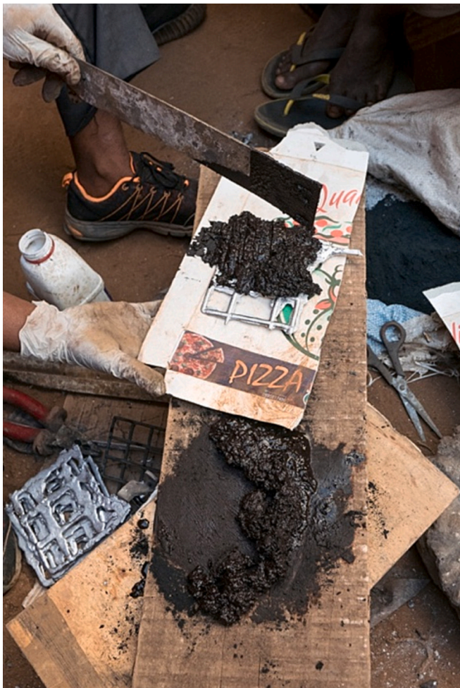
Fig. 2. Melted lead grids being coated in lead oxide paste to fabricate battery plates for a solar home system battery.
