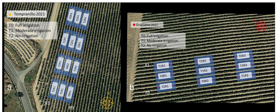
Figure 1. Experimental layout resulting a completely randomized block design with four replicates in (a) a Tempranillo vineyard plot, and (b) three replicates in a Graciano vineyard plot during season 2021. (This figure was prepared with QGIS 3.28.8 Firenze ( https://qgis.org/en/site/forusers/download.html ) using imagery available at IDE Rioja ( https://www.iderioja.larioja.org/index.php?id=8&lang=es ), with open access license CC BY).
