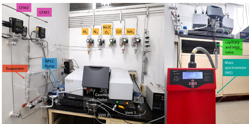
Fig. 3. System for operando measurements using diffuse reflectance infrared spectroscopy coupled to mass spectrometry (DRIFT-MS).
