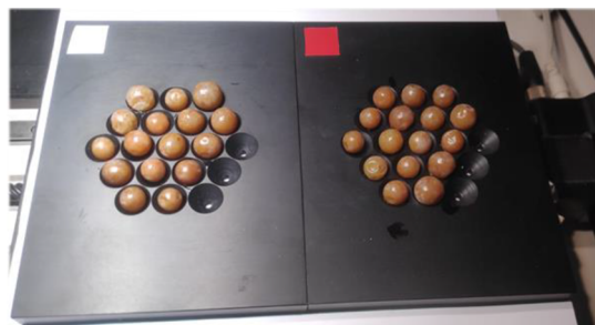
Figure 2. Fruit holders with the first subsample of 32 berries, 16 on each plate, prior HSI.
