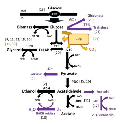
**Figure 1.** Diagram of the alcoholic fermentation pathway with indications of the steps affected by the different genetic modifications assayed to lower ethanol yields. References in black: genetic engineering. References in yellow: adaptive evolution. Metabolites outside of the central ethanol fermentation pathway are indicated in purple.
