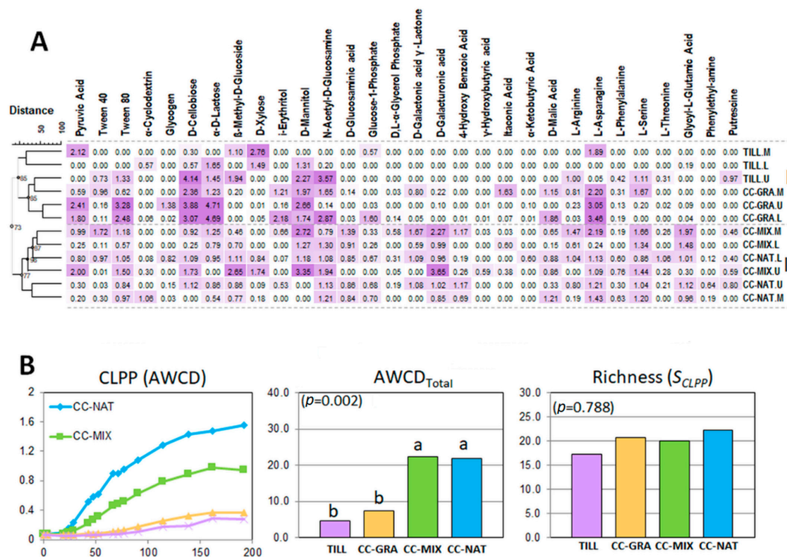
Figure 4. Carbon source assimilation profiles as measured by the Biolog EcoPlate™ of an olive orchard soil under different cover crop managements (TILL: tillage, CC-GRA: sown cover crop with gramineous and CC-MIX: sown cover crop with a mixture of species and CC-NAT (cover crop with spontaneous vegetation) and for each sampling point on the slope (U: upper, M: middle and L: lower). (A) Cluster analysis of combined data using the Ward algorithm applied to the similarity matrix generated from the community level physiological profiles (CLPPs) from absorbance readings at time 192 h by using the Bray–Curtis distance coefficient. Intensity of color in the figure is proportional to activity. Cophenetic correlation values are indicated in each node. (B) Kinetics of average well color development (AWCD) during the duration of the experiment and mean comparison of total AWCD (AWCD Total ) and total number of carbon source assimilated profiles at the end of the experiment (Richness, S CLPP ) was performed using the rank-based Kruskal–Wallis test and Dunn’s all-pairwise multiple comparison test was applied when appropriate ( p < 0.05 ). (Different letters indicate significant differences p < 0.05 .)
