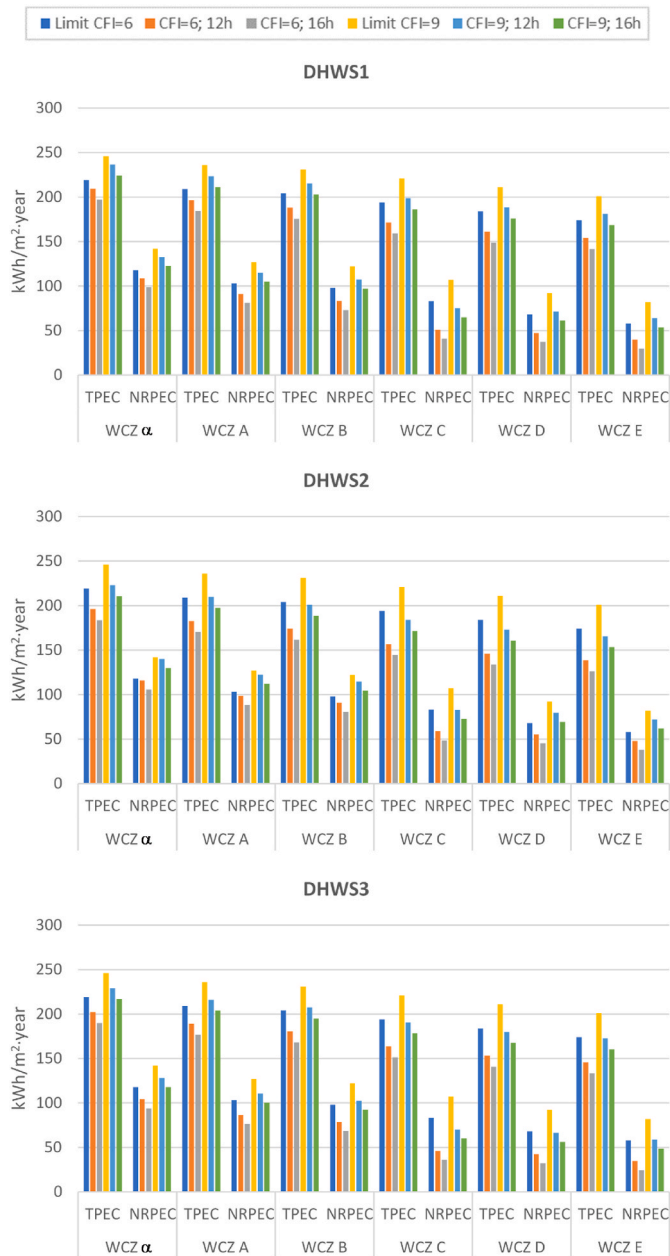
Fig. 18. Maximum possible TPEC and maximum possible NRPEC for heating, cooling, ventilation and humidity control services and the corresponding limit values for TPEC and NRPEC (in kWh/m 2 -year) for the proposed average internal loads, C FI , and occupancy periods for the non-residential buildings studied by DHW system and winter climate zone (WCZ).
