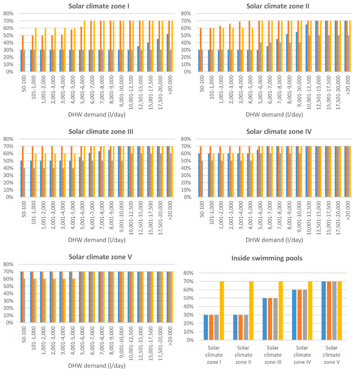
Fig. 4. Required minimum renewable energy contribution (in %) to meet part of the annual energy demand for DHW by DHW demand (in l/day) and for each solar climate zone and to meet part of the annual energy demand for the heating of indoor swimming pools by solar climate zone according to each CTE-DB-HE4 [42–48].
