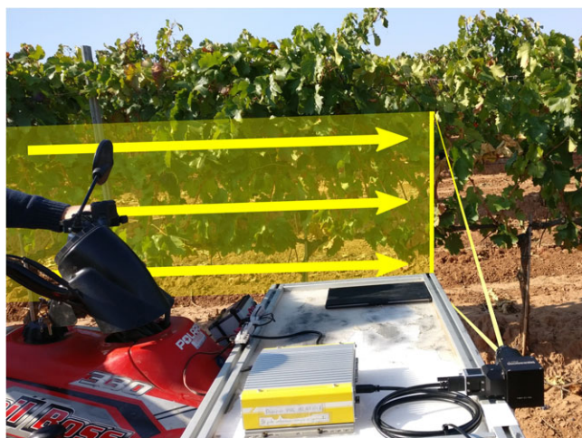
Figure 2. On-the-go hyperspectral imaging with a camera mounted on an all-terrain vehicle (ATV) at 5 km/h. Images of the entire vine canopy were obtained from the ATV's motion, by push-broom scanning, and used for the estimation of grape composition.
