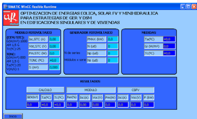
Figure 3: Screen of data introduction corresponding to the developed application of management of photovoltaic electric power in the building
