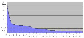
Fig. 2b Flow duration curve. Average year 2007.
