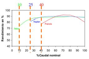
Fig. 1 Performance characteristic of different turbine types, applied the technical minimum flow.
