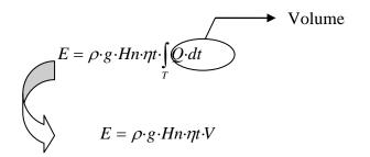
Function that determines that for obtaining maximum energy, turbines must harness the largest volume of water flowing through the river.
