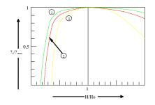
Fig 4. Performance characteristics depending on the head variation. (1) Kaplan; (2) Francis; (3) Pelton; Source [Vivier, L. 1966].
