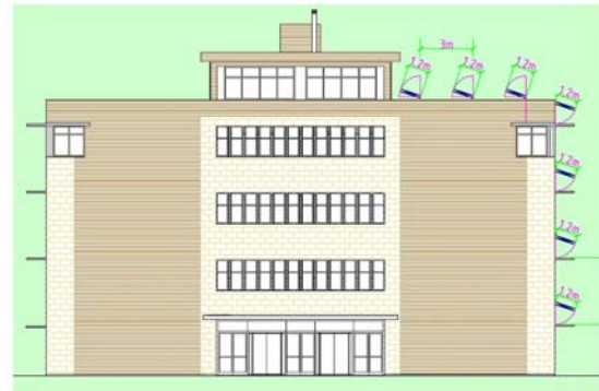
Fig. 03 Detail of an axis solar tracking on the south facade.
