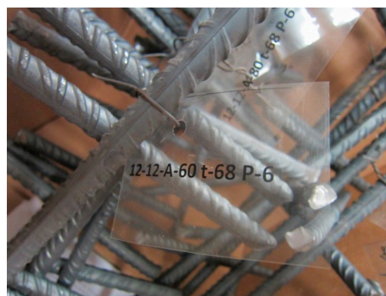
Figure 5. Label nomenclature of the joint thickness (12 + 12 = 24 mm).
