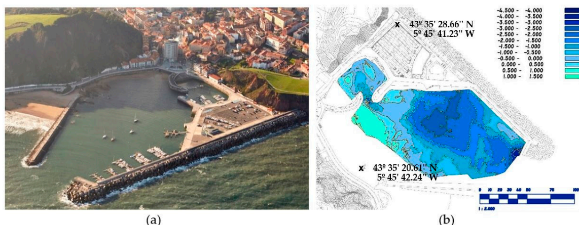
Figure 1. Study area (a) Candás port; (b) bathymetry using echo-sounding measurements. The colors denote the depth of the water in meters.
