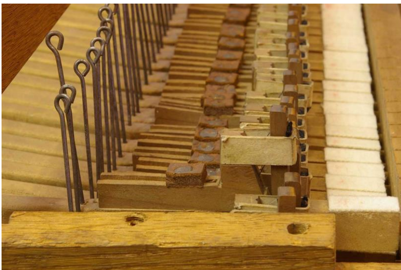
Figure 15. The 'adjustable escapement system' of the Clavecin royal No. 640 in Berlin (photo by Kerstin Schwarz).
