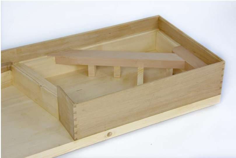
Figure 8. Case, dovetails and wrestplank of the facsimile (photo by Kerstin Schwarz).
