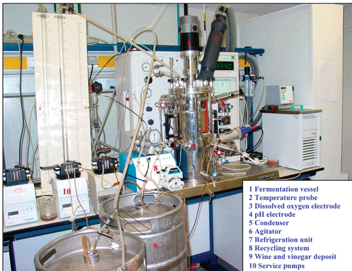
Figure 1. Pilot fermentation system.
