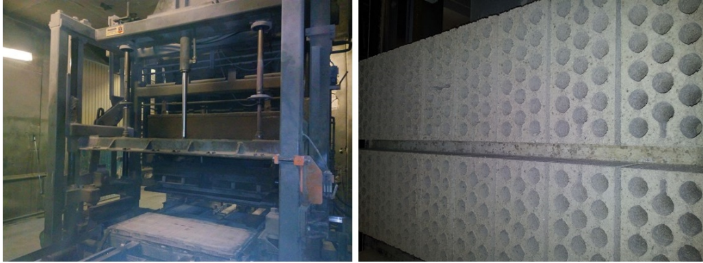
Figure 2. Brick manufacturing: compacting unit (left); and tray conveyor (right).
