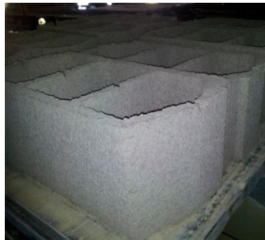
Figure 3. Hollow block manufacturing.
